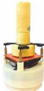
Left: a cell in which the R.H. & T can be maintained. Right: a custom-made cell able to perform freeze-thaw cycles (De Schryver et al. , 2016)
